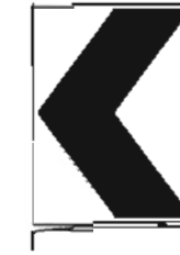
18" x 24" Sign (Maximum Sign Dimension) Chevron CM-8, Opposing Traffic Lane Divider, Driveway sign D70a, Keep Right R4 series or other signs as approved by Engineer
