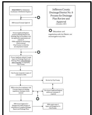
Figure G - JCDD6 Process for Drainage Plan Review and Approval
